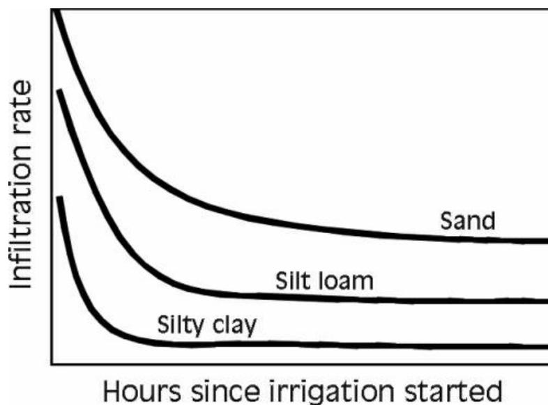
**Figure 3.7. Typical infiltration curves for different soil textures.**
