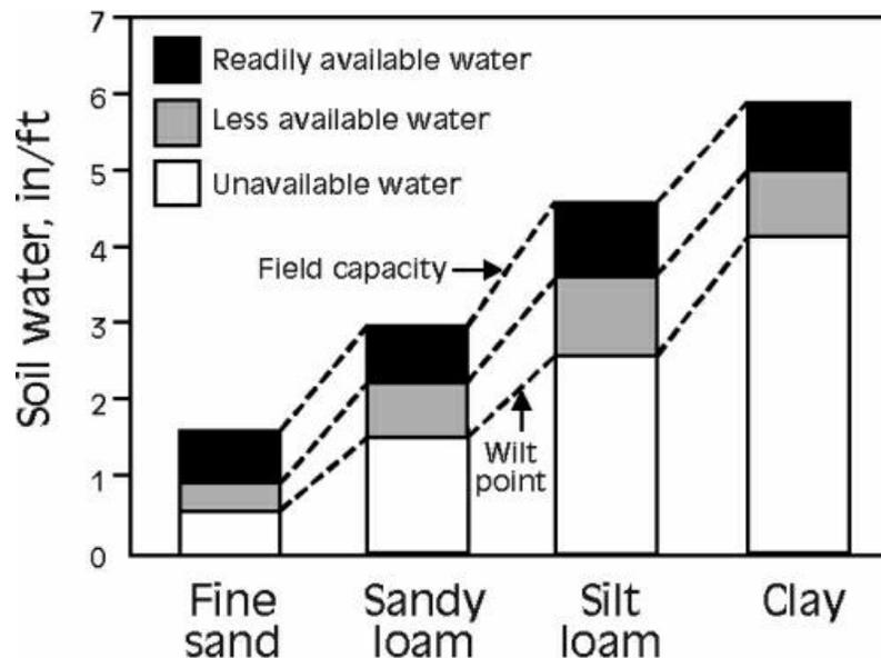
Figure 3.5. Soil water components in four common soil types.
