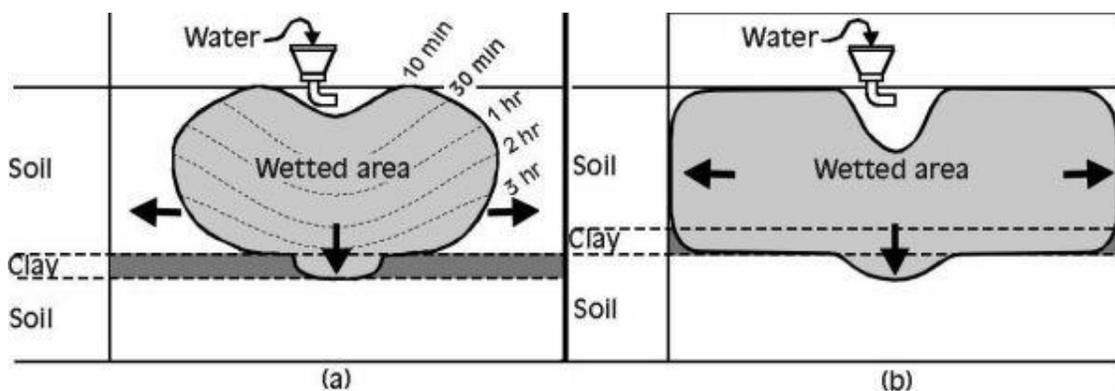
**Figure 3.9. Water infiltrating into soil underlain by clay layer.**
