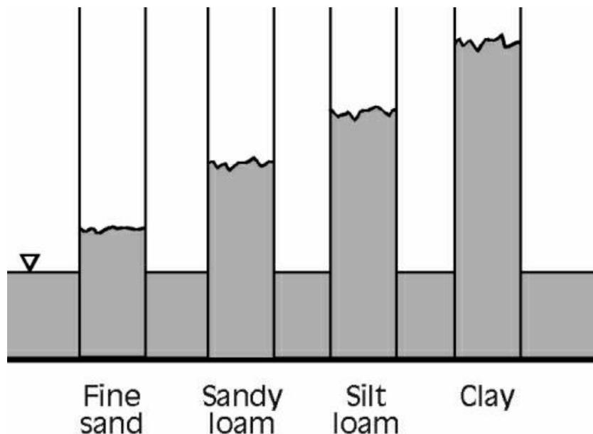
**Figure 3.4. Capillary action illustrated by the relative height of wetting for four soil textures.**
