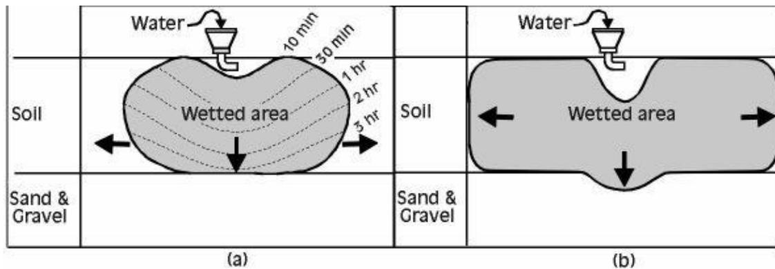
**Figure 3.8. Water infiltrating into soil underlain by coarse sand and gravel.**
