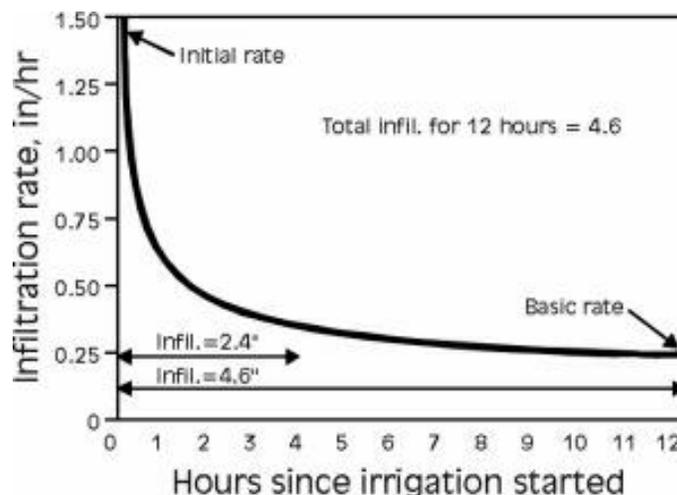
**Figure 3.6. Typical infiltration curve for Hastings silt loam soil.**
