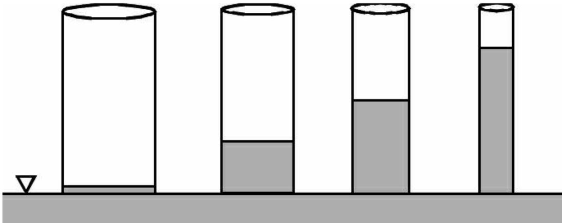
**Figure 3.3. Capillary action is illustrated by how far water rises in tube of various diameters.**
