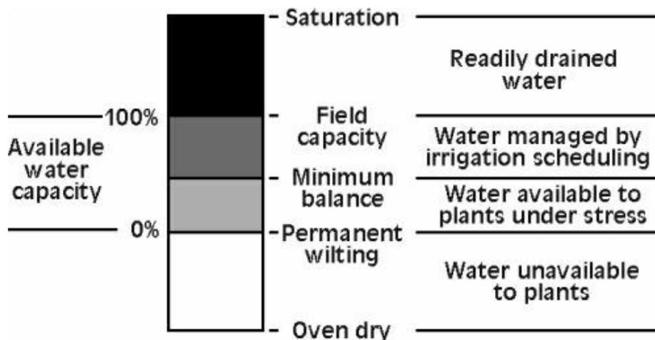
**Figure 3.2. Components of the soil water reservoir.**
